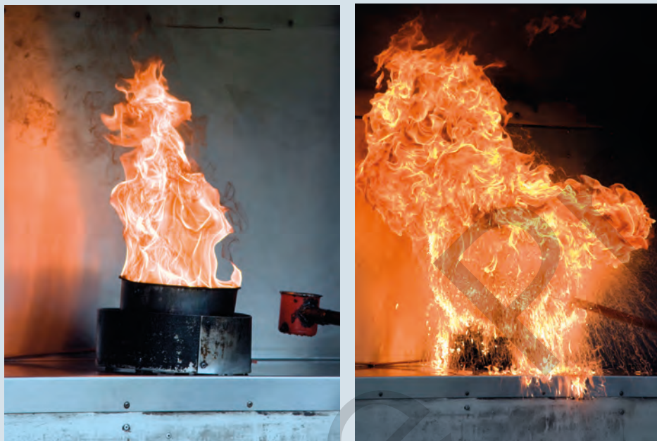
FIGURE 1.2.3 Using water on a fat, oil or grease fire can accelerate the rate of a combustion reaction with life-threatening results.
